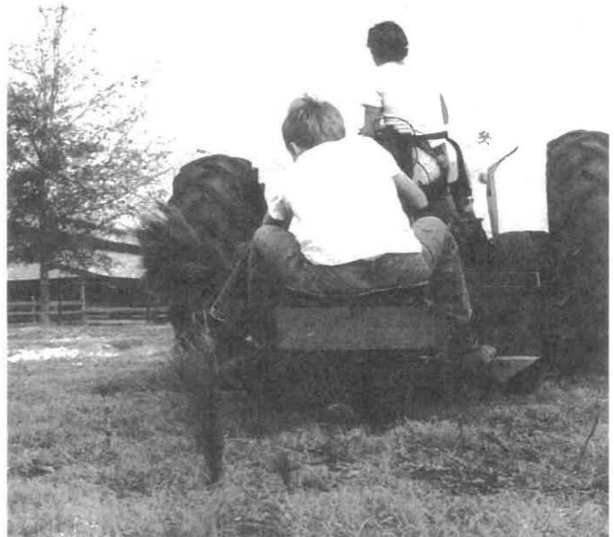
This tractor-powered mechanical planter operated by Billy Mann (driver) and Randy Fox digs a furrow then covers it up after pine seedlings have been dropped at intervals. Apprentice planter Paul Hutto watches the procedure.
