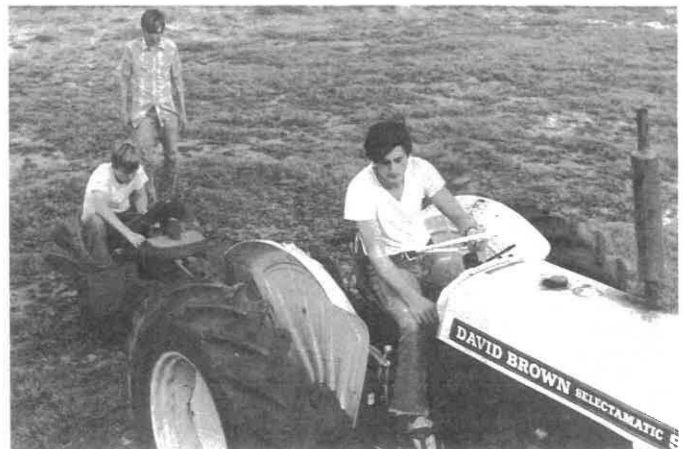
This tractor-powered mechanical planter operated by Billy Mann (driver) and Randy Fox digs a furrow then covers it up after pine seedlings have been dropped at intervals. Apprentice planter Paul Hutto watches the procedure.
